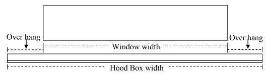
The left hand screw for the Hood Box should be places to the left of the top corner of the window at the attachment point of the over hang and 180mm higher (the height of the Hood Box). If installing on a brick wall NEVER put the screw into a mortar line. If the position you need to drill is over a mortar line move up to the bottom of the brick above that position.
