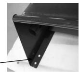
Hang the left tab of the hood box over the screw. Lift the right side of the Hood Box so it is level with the top edge of the window. Mark where the right hand screw will go. Take the Hood Box off the window. Insert your right hand screw, again leaving about 15mm out for the Hood Box to hook onto. Hang the Hood Box on the screws. Fasten the screws tighter. Drill and secure the bottom of the Hood Box each side through either of the lower inside holes that are not on a mortar line.
