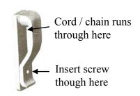
Ensure that there is SUFFICIENT TENSION on the chain/cord – however excessive tension will impair smooth operation of the blind. Hold the Tension Device in the correct position, as shown. Insert and secure the screw through hole. Make sure the screw is affixed into a solid surface.
