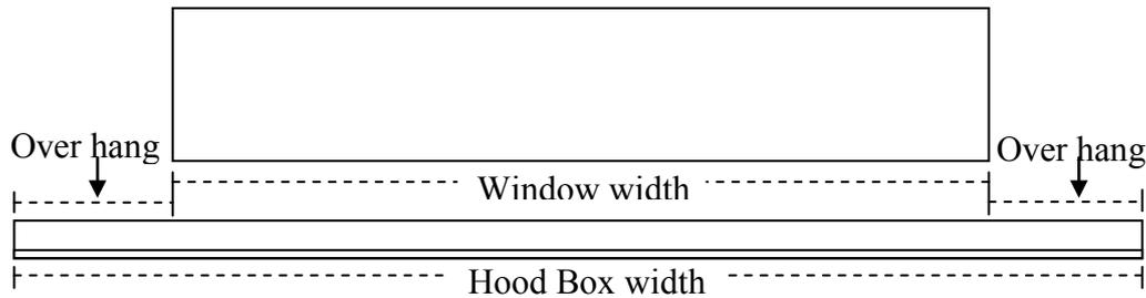
The left hand screw for the Hood Box should be placed to the left of the top corner of the window at the attachment point of the over hang and 180mm higher (the height of the Hood Box). If installing on a brick wall NEVER put the screw into a mortar line. If the position you need to drill is over a mortar line move up to the bottom of the brick above that position.
